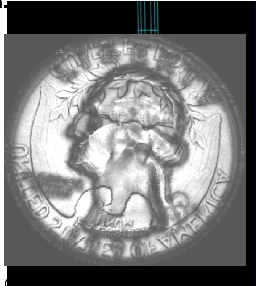
Gray scale image produced using the sound reflected from the back surface of the coin (inspected from "heads" side)
